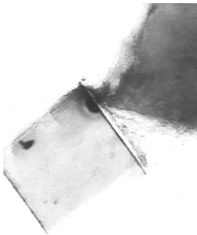
Fig. 8 Welding fume consisting of aluminium particles with an oxide layer. A stress field is observed at one of the contacts
