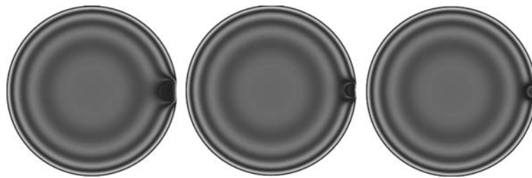
Fig. 20 Simulated contrast from the stress field of a coherent particle lying with its centre at the contacting point between two particles. The particle radius (of the large particles) is 1.1 \times 10^{-7} m.
